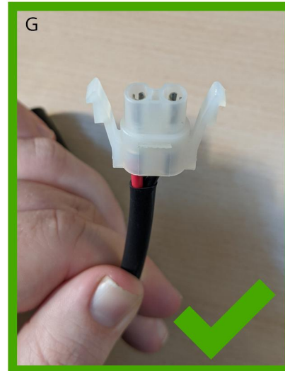
(G - J) Multiple angles of the connector are needed to help determine the correct connector. (J) A clear photo of how the wires, from the battery, fit into the connector is important to ensure correct polarity.
