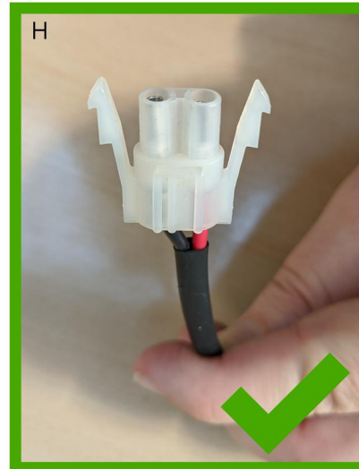
(G - J) Multiple angles of the connector are needed to help determine the correct connector. (J) A clear photo of how the wires, from the battery, fit into the connector is important to ensure correct polarity.
